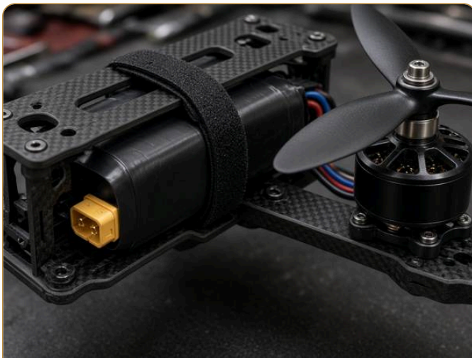
Concept render: 6S 21700 Li-ion pack (XT60) and 2807 motor with 7-inch prop
