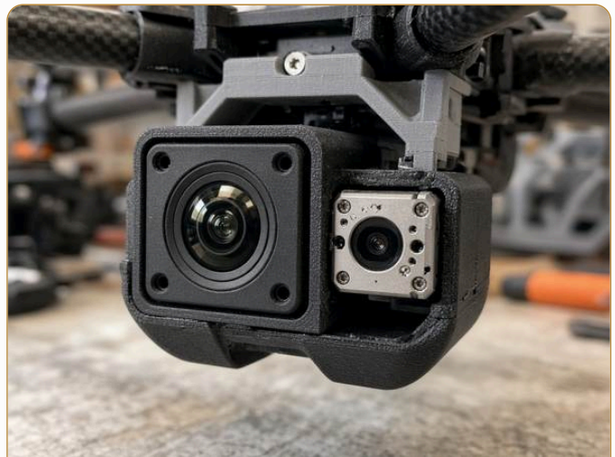
Concept render: recording pod, Camera Module 3 plus optional thermal module
