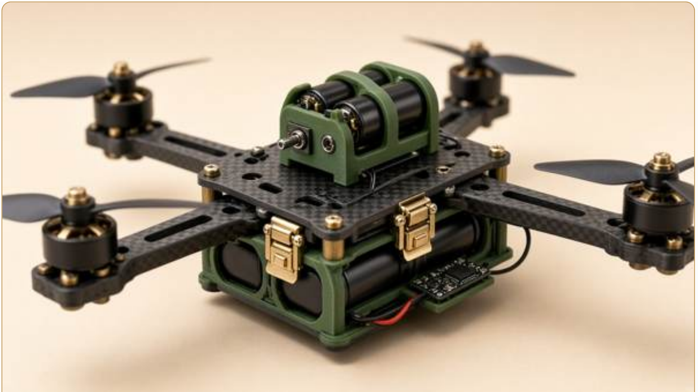
Concept render: 2S 18650 brain pack with switch and charge port on the top plate; motor pack on the quick-swap under-sled
