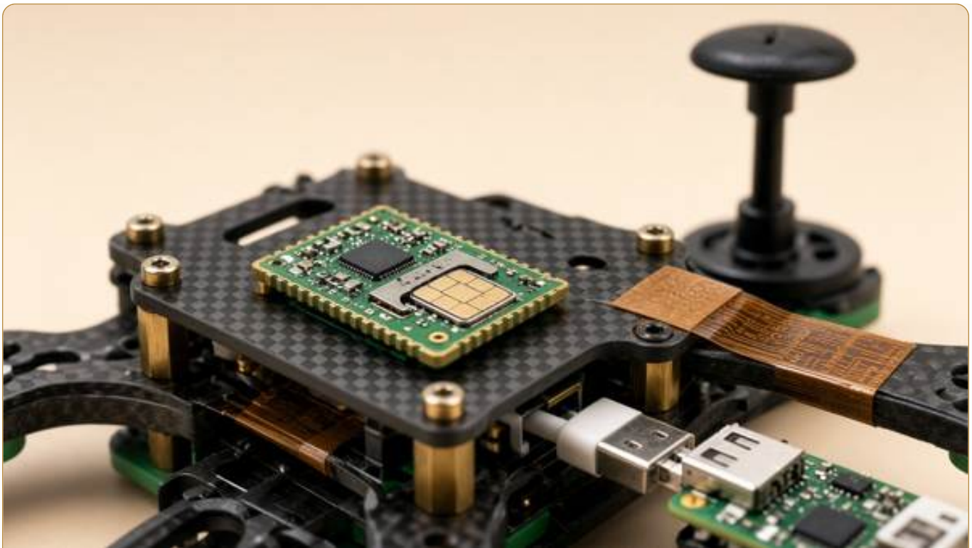
Concept render: LTE-M module with nano SIM on the top plate, flex FPC antenna run out along an arm away from the GPS mast
